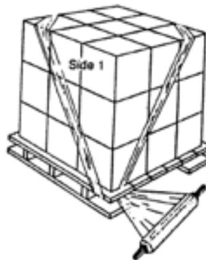
Diagram 5: Pull roll down and catch on pallet.
