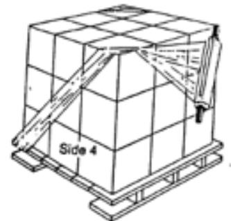
Diagram 4: Pull roll down and catch on pallet.
