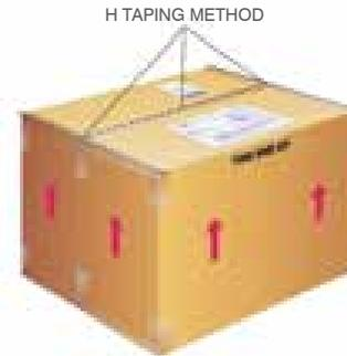
Non-packaging tapes such as masking tape, duct tape, cellophane and other such tapes should not be used as a substitute for quality box sealing tape.
